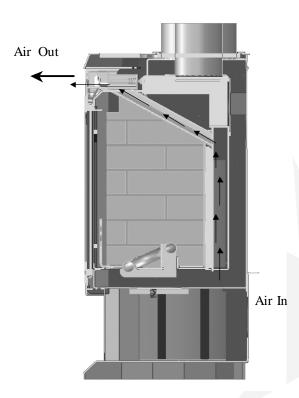
The flow of combustion and ventilation air must not be obstructed.
